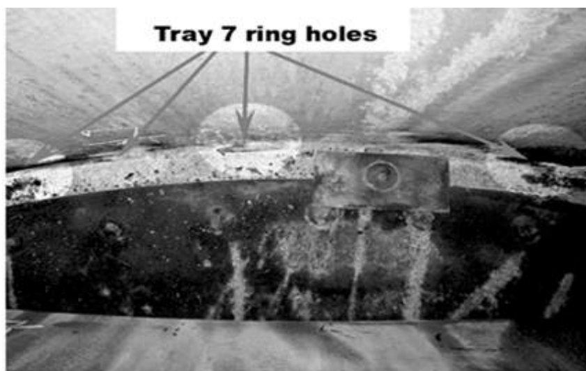
Figure B.89—Tray Support Ring Corroded to Failure
