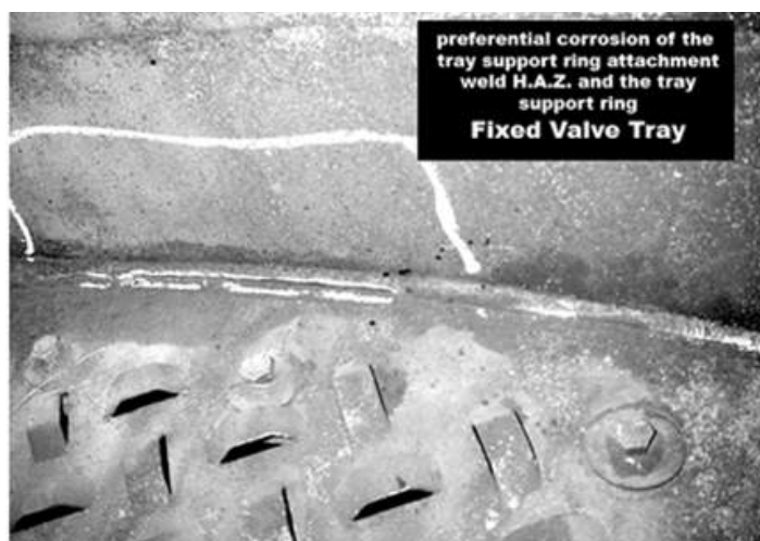
Figure B.77—Small Fixed Valves
