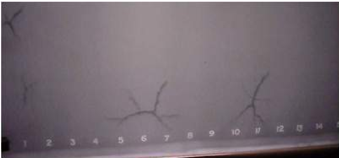
Figure 20—Radiograph of Self-vented Hydrogen Blisters in Carbon Steel
