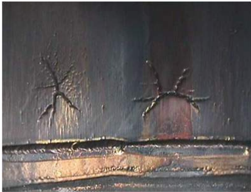
Figure 19—Self-vented Hydrogen Blisters
