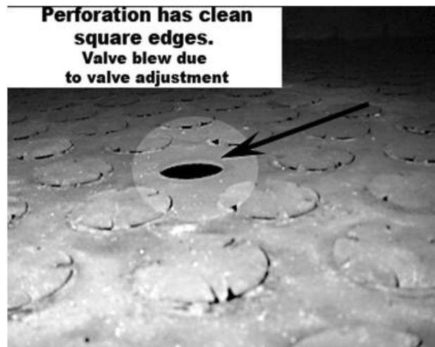
Figure B.70—Clean Square-edged Perforation
