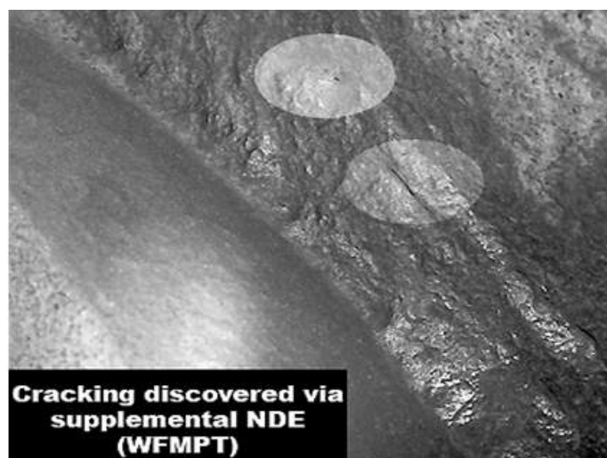
Figure B.64—WFMPT Discovered Cracking
