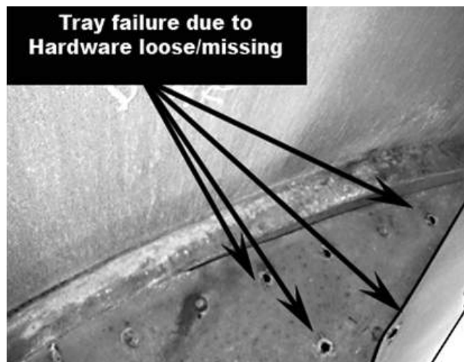
Figure B.86—Loose and Missing Hardware Failure
