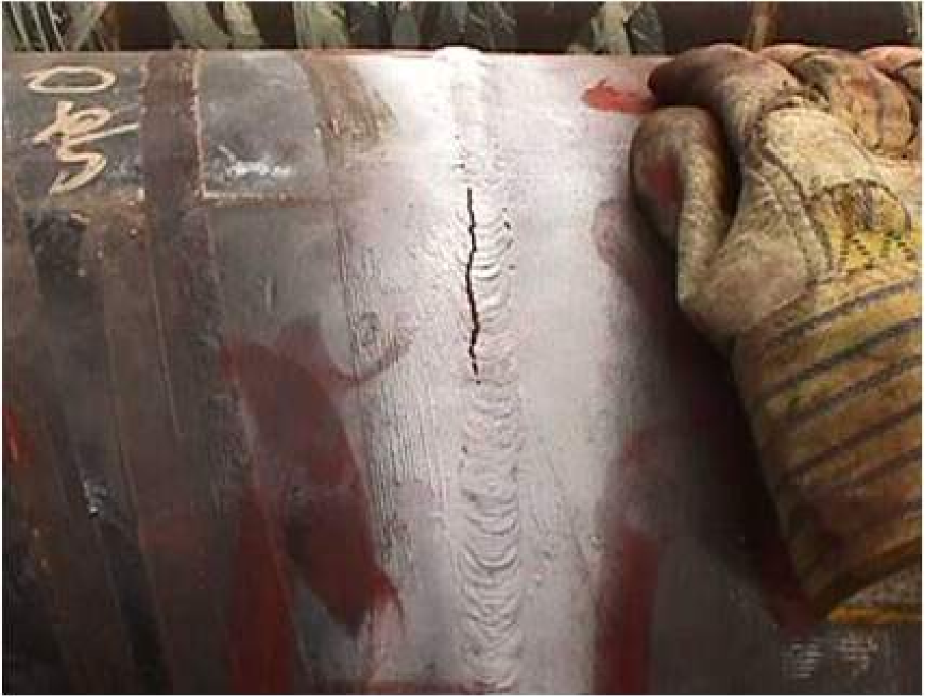
Figure 17—Crack in Weld Seen by PT
