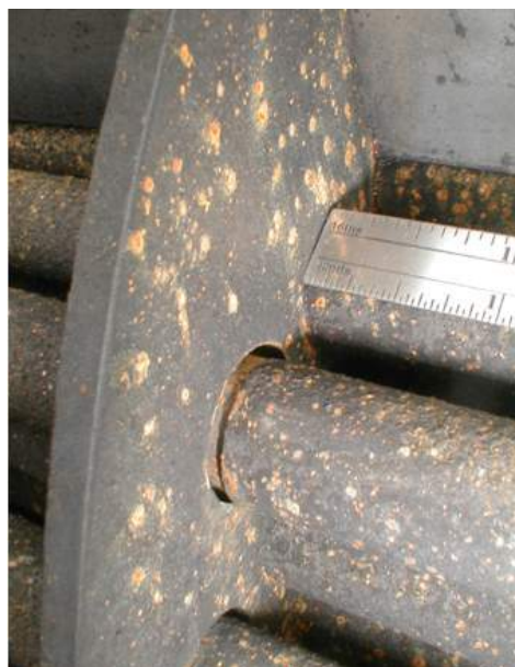
Figure A.8—Tubes Thinned at Baffles
