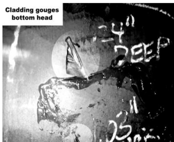
Figure B.60—Cladding Breech at Gouges in Bottom Head
