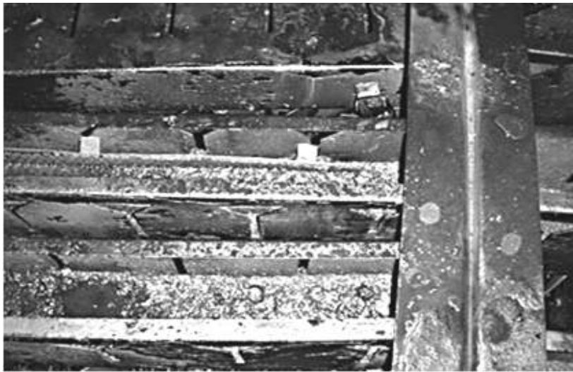
Figure B.46—Fouled Troughs on Box and Trough Distributor
