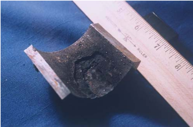
Figure 13—Localized Tube Wall Loss Caused by Caustic Gouging
