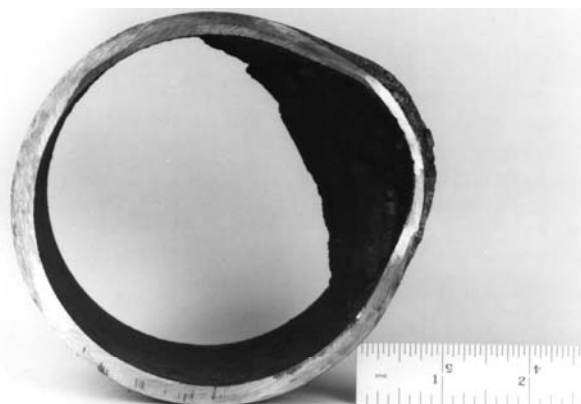
Figure 15—Short-term Boiler Tube Failure Caused by Waterside Deposits, Subsequent Overheating, and Final Bulging of the Tube Wall
