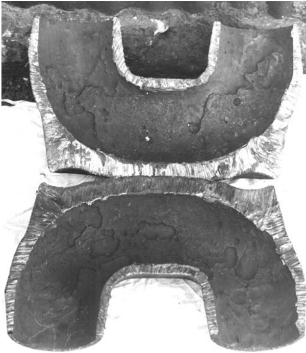
Figure 26—Corrosion of U-bends
