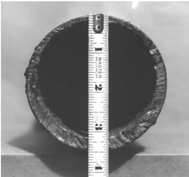
Figure 29—Eccentric Corrosion of a Tube
