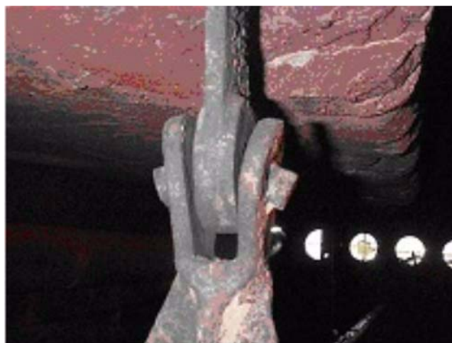
Figure 35—Yielding and Creep of a Tube Support Connection
