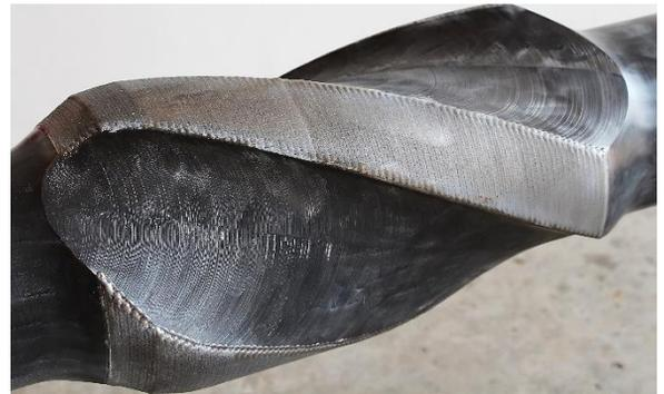
Laser cladding and coating yield high precision and homogeneity in depositing powder onto the base material. The coatings and overlays impart greatly improved performance of the desired characteristics such as: wear resistance, impact resistance, sliding wear, corrosion protection, friction modification and specific electrical properties.
