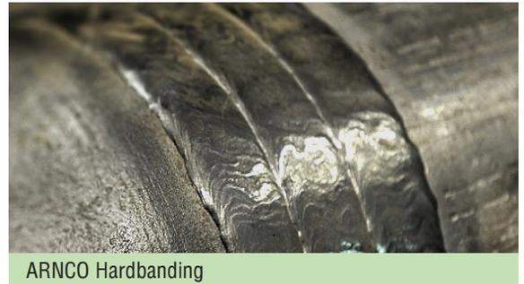
Precisely controlled pre-heat and post-heat conditions ensure that only fully-metallurgical bonded hardbanding overlays of optimum integrity are applied. The deposit is made flush to + 1/32 above the O.D. of the collar.
