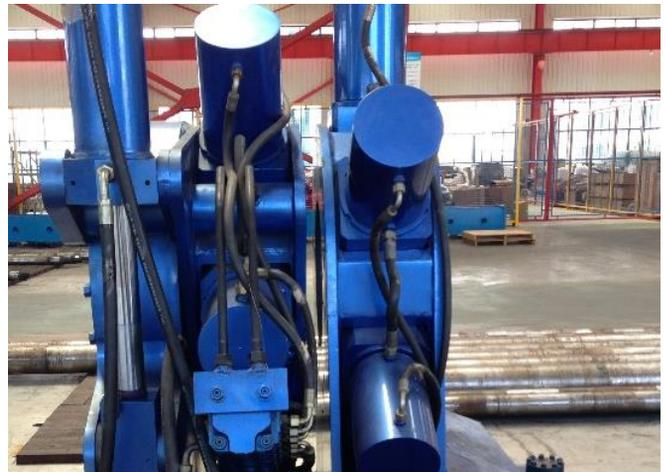
Screwing Tong Rotary Device
