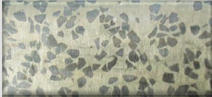
Crushed Tungsten Carbides are fused together within a tough polycrystalline matrix of nickel. The 3mm grain size ensures greater concentration of carbide which is ideal for soft formation drilling.
