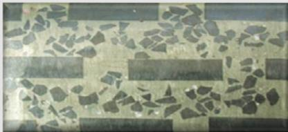
In this hard-facing, trapezoidal tungsten carbide inserts are held in a sintered carbide nickel bronze matrix. This will give a greater depth of carbide coverage – ideal for high deviation drilling in abrasive formations.
