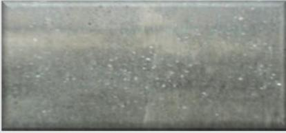
**(Flexicoy Technodur):** Fused tungsten carbide in a nickel chrome boron matrix designed for oxy-acetylene torch application and available for components subject to high levels of wear. Flexicoy has pure nickel core surrounded by fused tungsten carbide and alloy elements for the matrix. This fused together when deposited to form a tough wear resistance surface.
