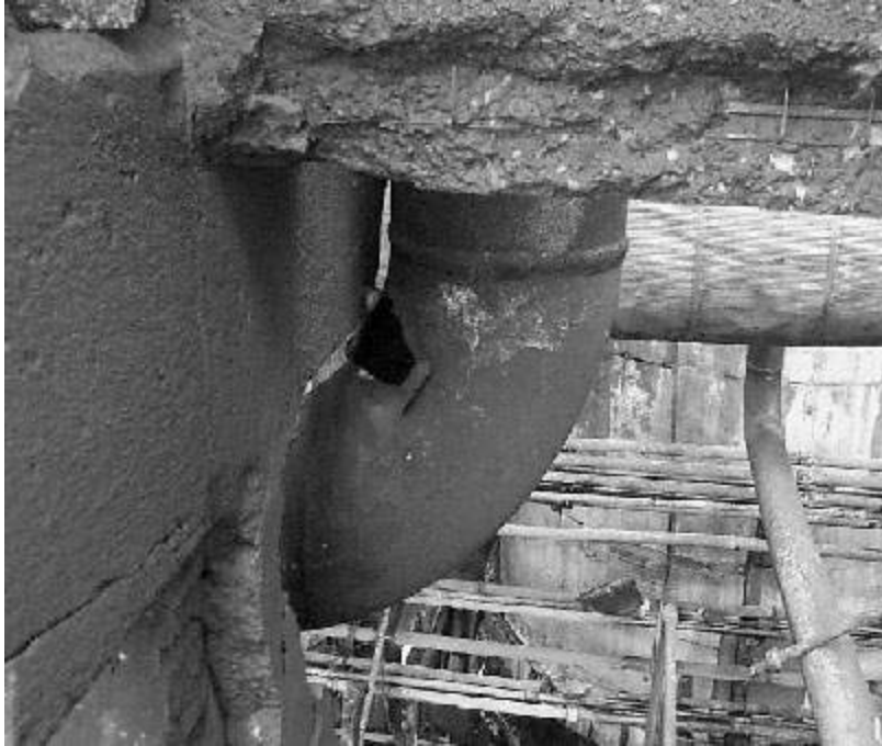
Figure 4-120 – Sulfidation failure of piping elbow.
