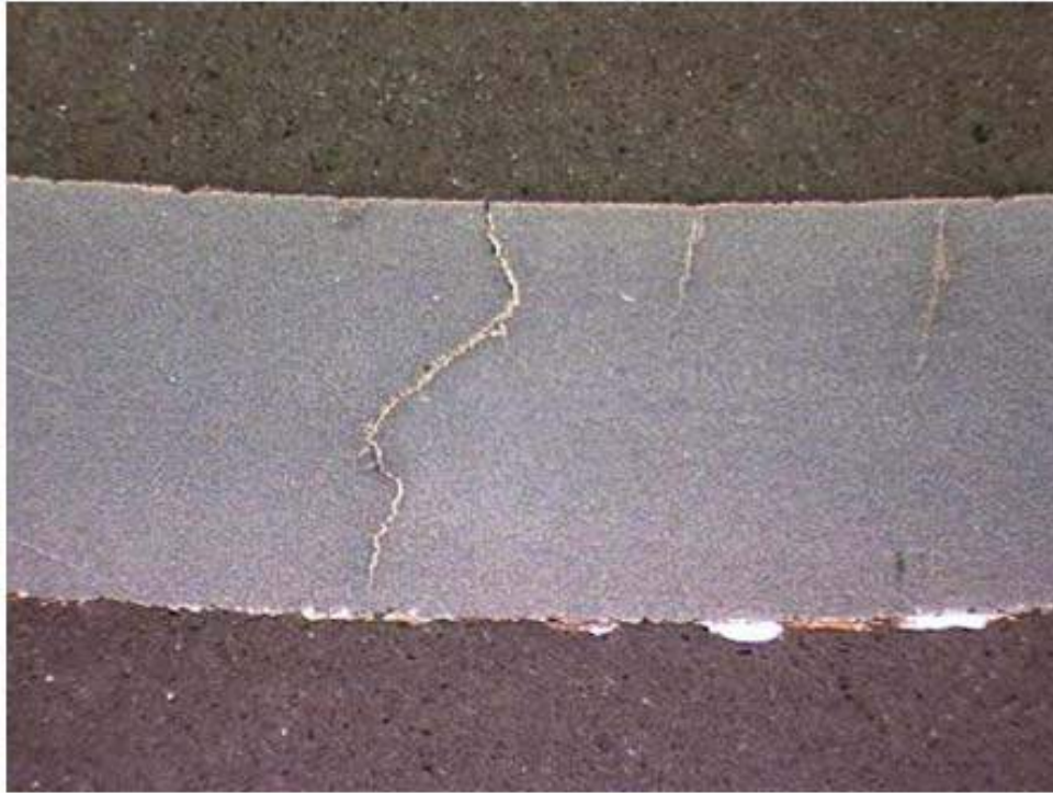
Figure 4-168 – Transverse cross-section of a piping section exposed to fuel ethanol showing multiple crack initiation sites characteristic of SCC.
