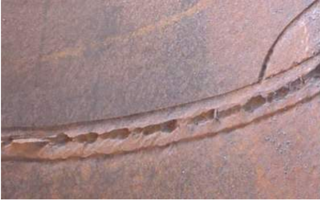
Figure 5-3 – Preferential weld corrosion in lean amine (Reference 5)
