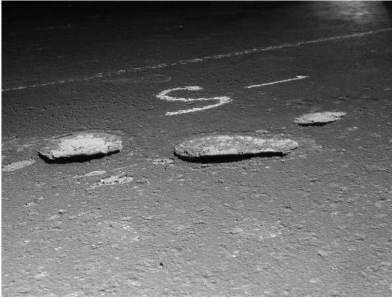
Figure 4-89 – MIC of diesel tank bottom.
