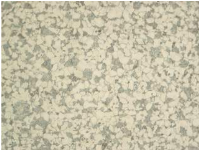
Figure 5-58 – A photomicrograph of the outside surface of a pipe section, shown in the previous figure, exhibits a normal ferritic-pearlitic structure. Mag. 200X
