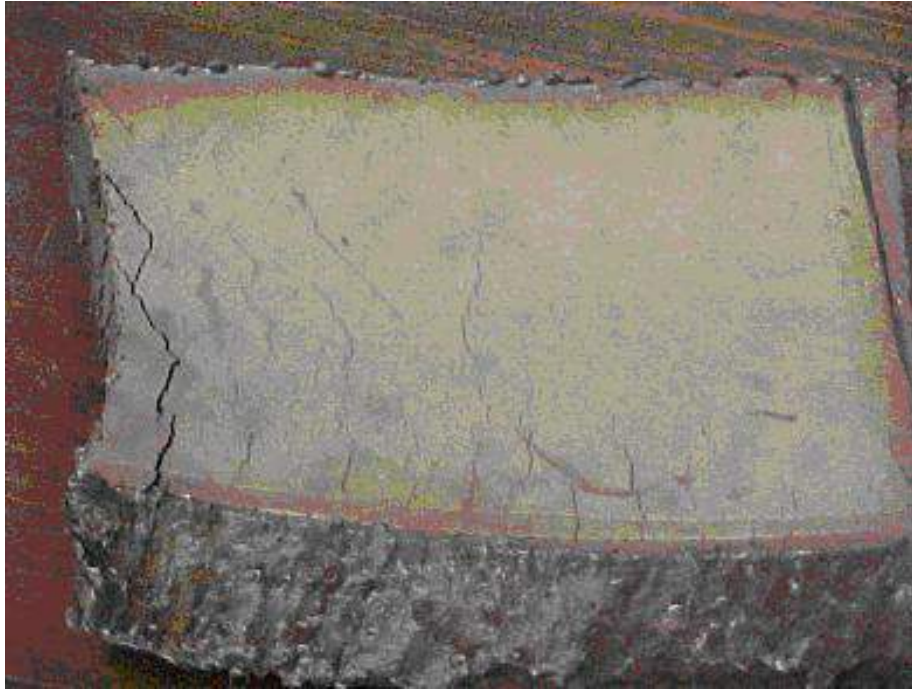
Figure 4-20 – Thermal fatigue cracks on the inside of a heavy wall SS pipe downstream of a cooler H 2 injection into a hot hydrocarbon line.
