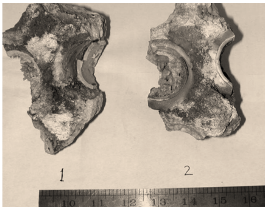
Figure 4-59 – Damaged refractory and ferrules.
