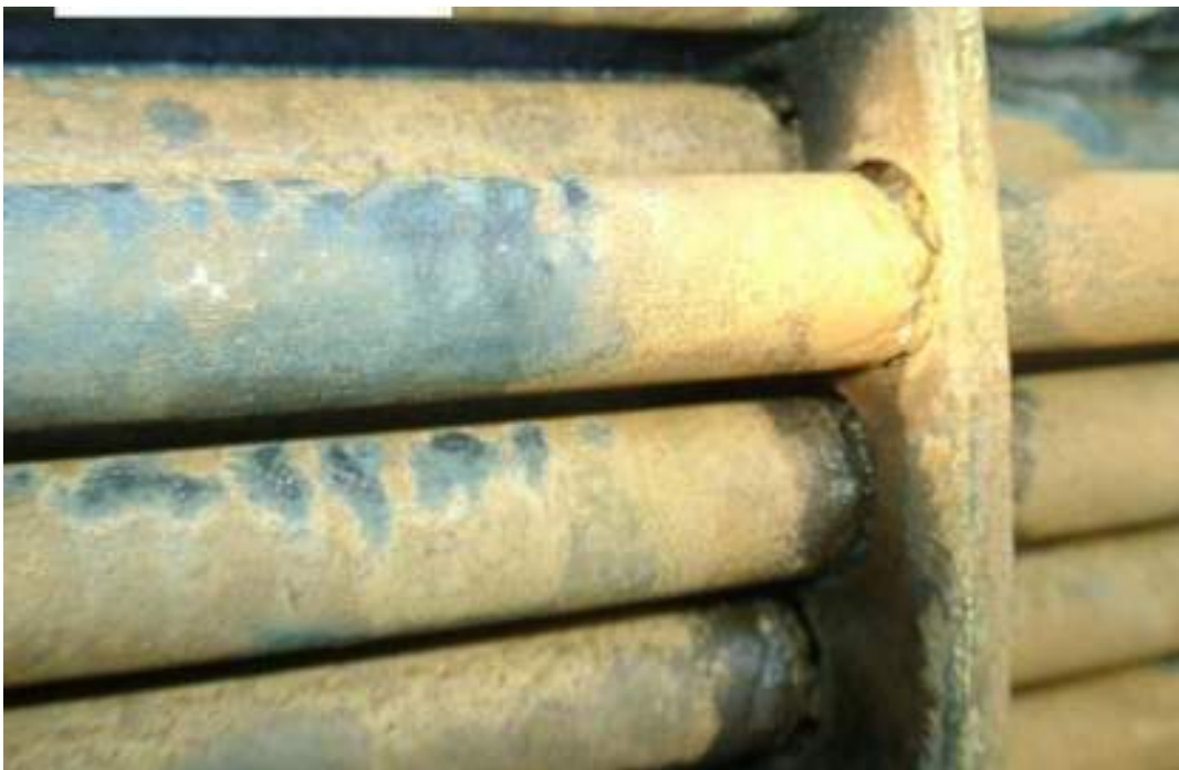
Figure 5-22 – Accelerated corrosion under a baffle.
