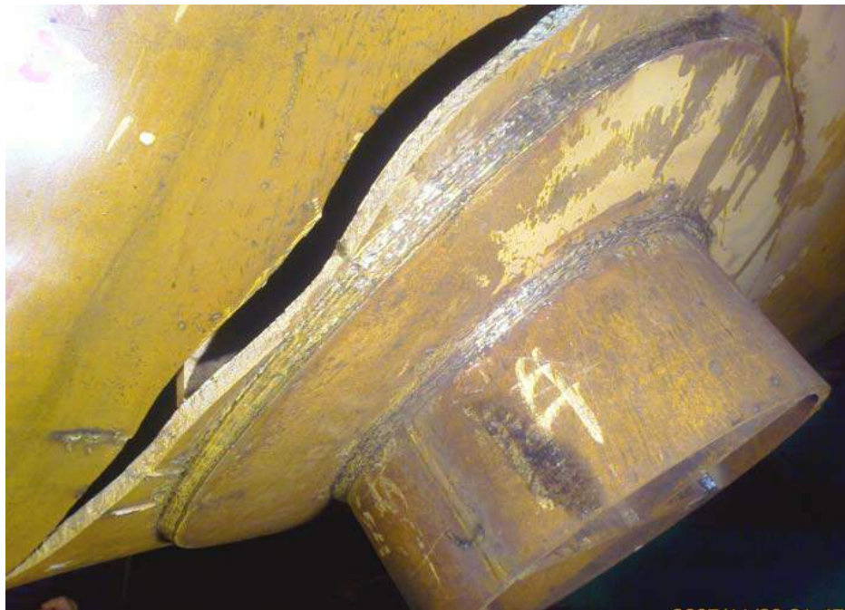
Figure 4-15 – Brittle Fracture of vessel shell during hydrotest.
