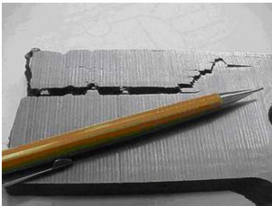
Figure 5-36 – Cross-section of plate showing HIC damage in the shell of a trim cooler which had been cooling vapors off a HHPS vessel in a hydroprocessing unit.
