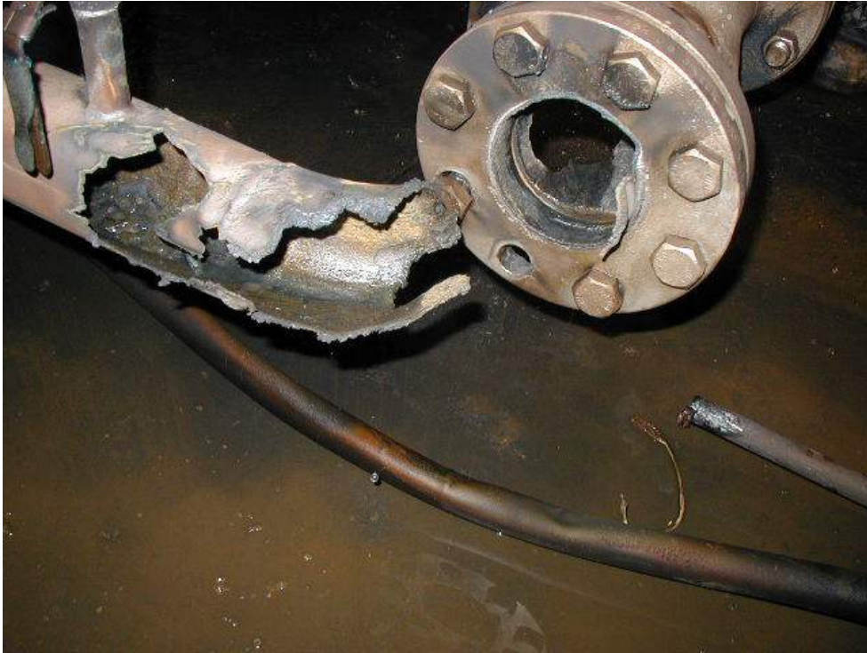
Figure 4-67 – Photograph of a burned 304 SS elbow. The fire started in an upstream stainless steel wire filter (due to particle impact) and the burning filter material impacted the elbow and ignited it. Thin stainless steel components (e.g., filter) are much more flammable than thicker SS. Thin SS (<1/8") is usually avoided in oxygen systems.
