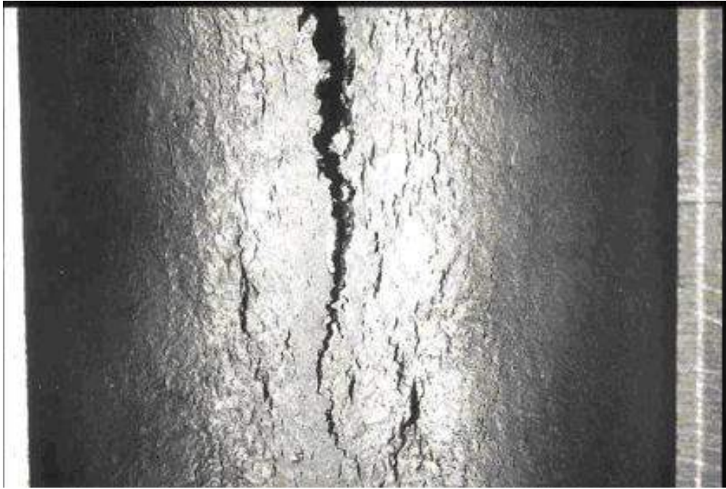
Figure 4-18 – Creep rupture of an HK40 heater tube.
