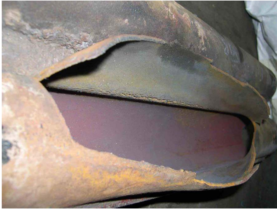
Figure 4-141 – Corrosion fatigue failure of a boiler tube.
