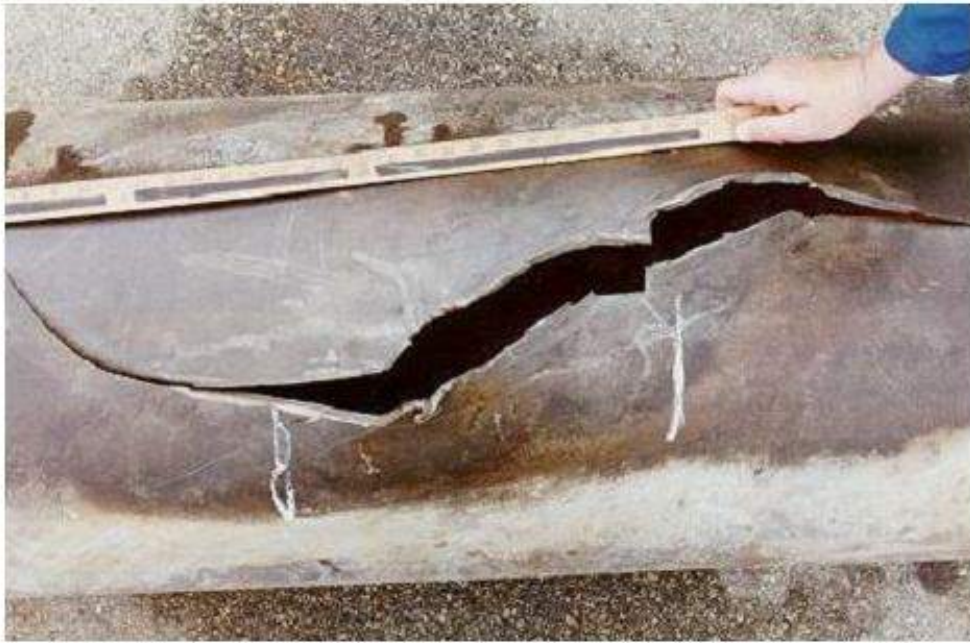
Figure 4-12 – 20-inch carbon steel pipeline that failed during hydrotest at gouges on the O.D.
