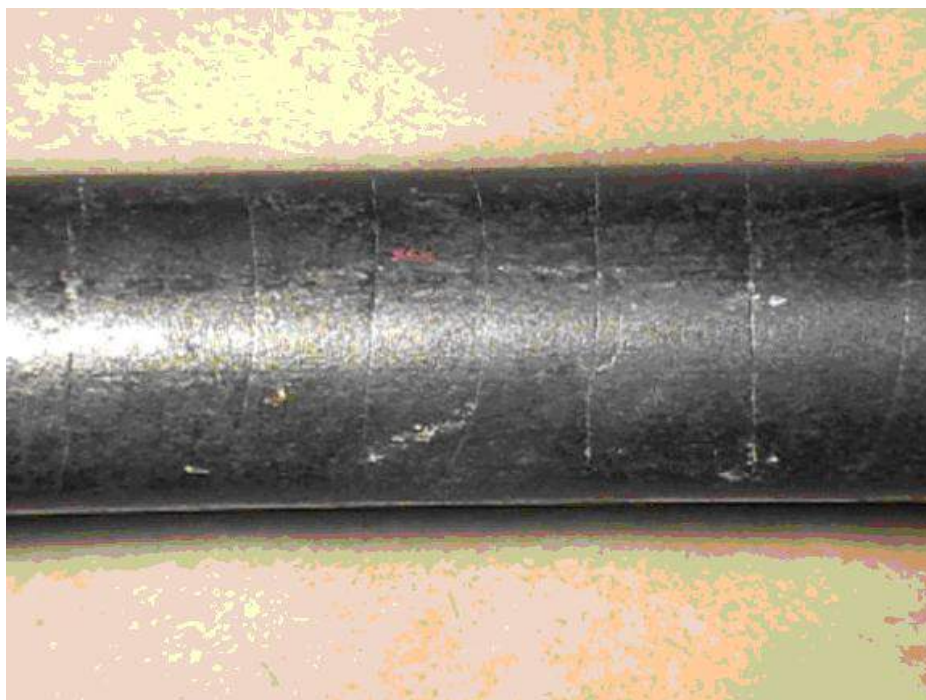
Figure 4-130 – A nitrided 5Cr-0.5Mo thermowell from an ammonia synthesis plant with surface cracking.
