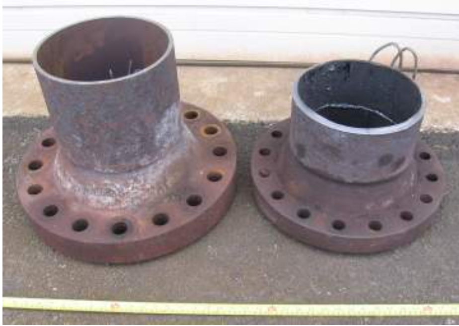
Figure 5-57 – A pair of 10 inch Carbon-0.5Mo flanged pipe sections (SA335-P1 & SA234-WP1) from a hot bypass line in a catalytic reformer that was designed to remain closed but operated partially or fully open for unknown lengths of time. They were in service for ~34 years at temperatures up to 960°F (516°C) and a hydrogen partial pressure of 198 psig (1.37 MPa).
