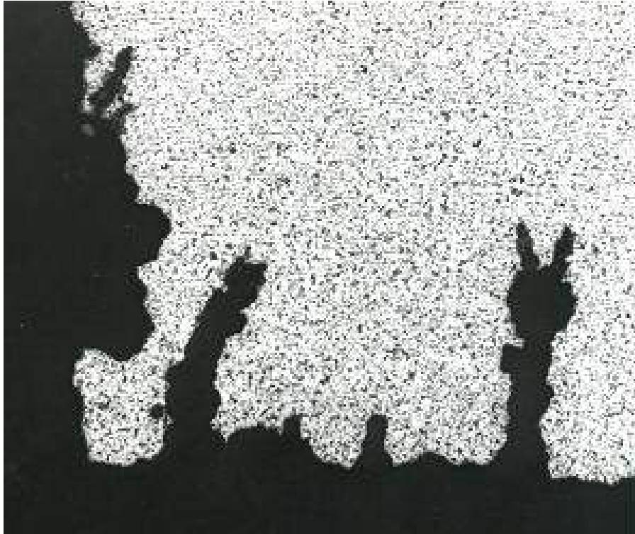
Figure 4-145 – Photomicrograph showing the crack morphology that is rounded with multiple lobes, and may branch to form “rabbit ears.” (Mag. 25X, etched.)
